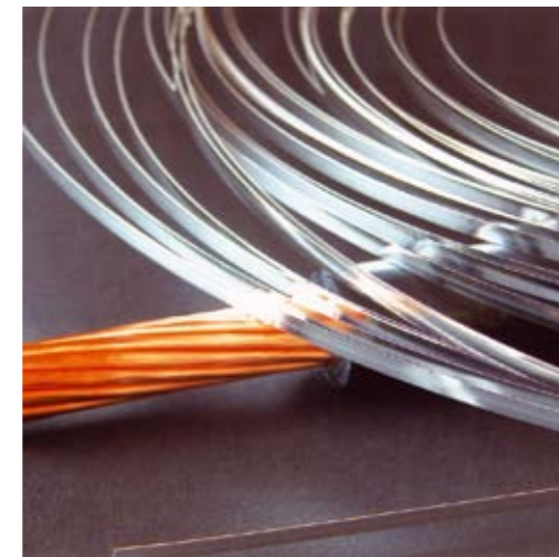
Superconductor compared with conventional copper cable.
