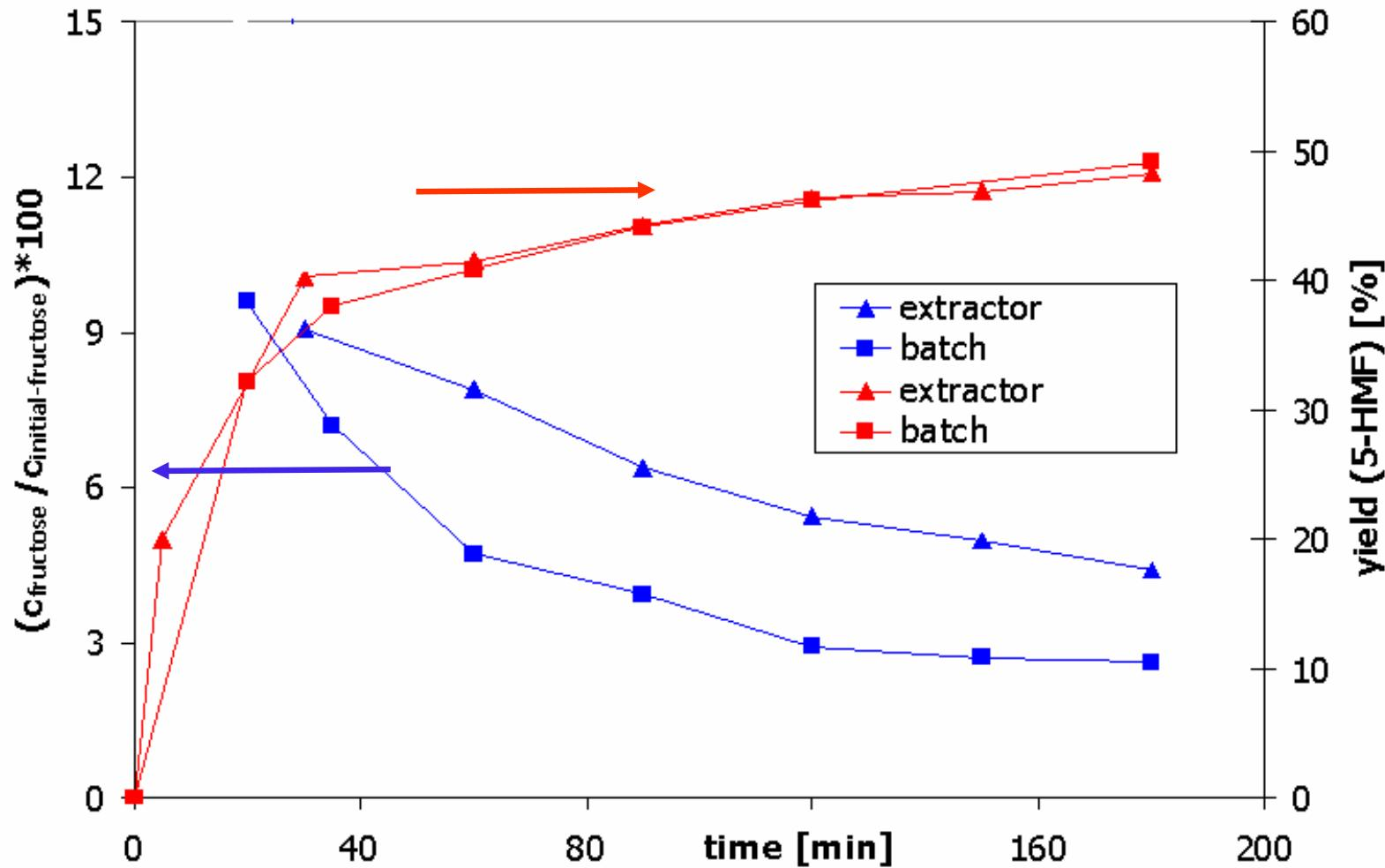
5.0 g (batch)/ 300.0 g (Reaktivextraktion) [ $C_4mim][CH_3SO_3$ ] (2 wt.% MSS), 17.2 wt.% Fructose, 80 °C
