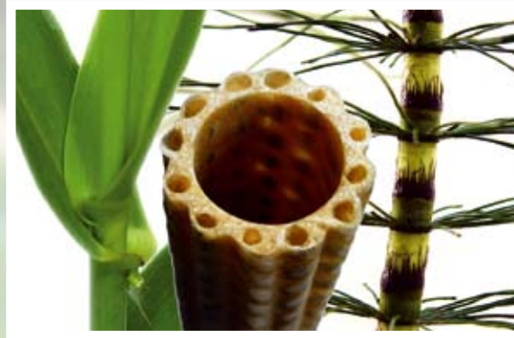
Technical Plant Stem modelled on the Gigant Reed and Horsetail. (© Plant Biomechanics Group Freiburg)
