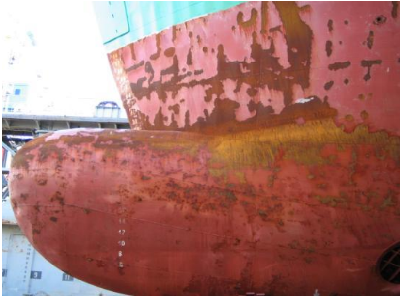
Conventional paint system after 18 months
