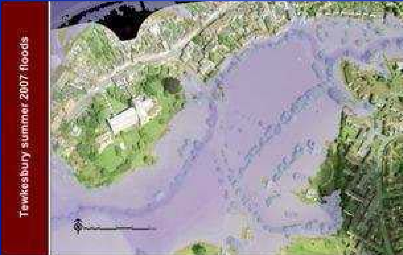
LISFLOOD-FP model using LiDAR data at 2m resolution. Image © Paul Bates, University of Bristol.
