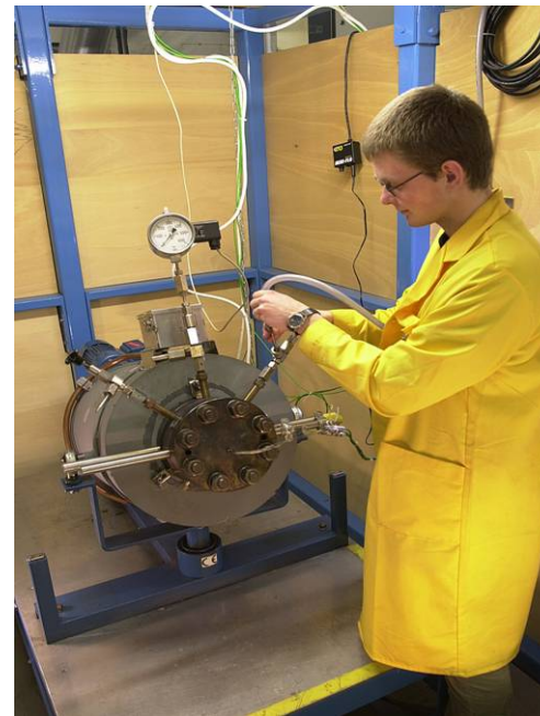
Tumbling batch reactor 500 °C, 50 MPa, 1 L
