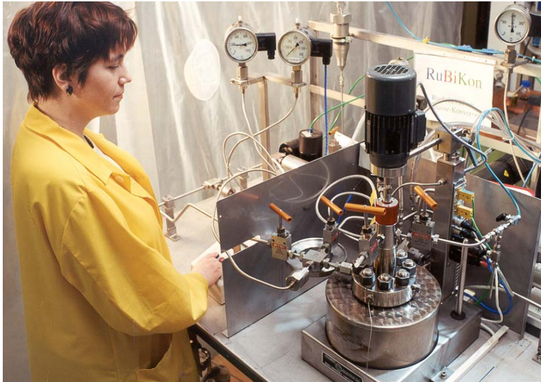
Tumbling batch reactor 500 °C, 50 MPa, 1 L
