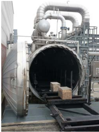
93 m 3 industrial batch thermolyser reactor
