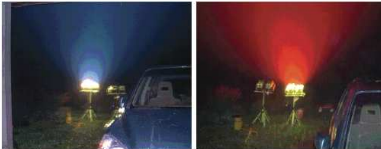
Figure 1. 1500W halogen test lights with blue and red filters used to study the impact of light upon migrating birds.
